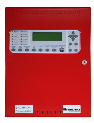
The FireNET Plus® 1127 series control panel is an intelligent addressable fire alarm panel with options containing 1 or 2 SLC loops. The panel supports any combination of addressable devices, up to 127 per signaling line circuit, including thermal and photoelectric smoke detectors/sensors, and monitoring and control modules. The Loop Explorer Windows® based software interface provides the installer with fingertip access to installation programming and diagnostic tools.
